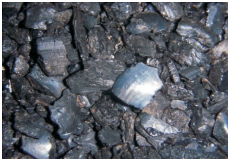
图 7 AHDEB 油田白垩系油藏钻遇的沥青 Fig.7 The asphalt in Cretaceous reservoirs of AHDEB oil field
