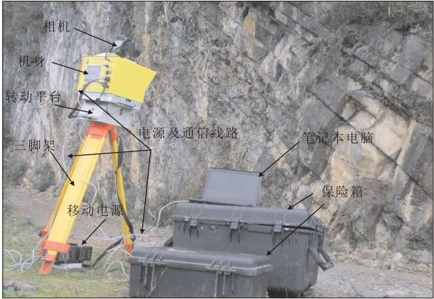
图 2 ILRIS-3 s D 型三维激光扫描仪安装示意 Fig.2 The field set up of 3-D laser scanning to measure geometric information of rock discontinuities
