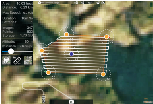
图 4 研究河段无人机航线规划 Fig.4 UAV flight planning for the study reach
