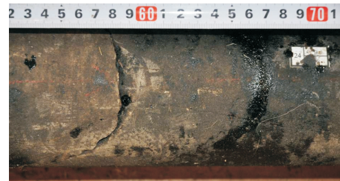
图 7 吉 C 井云质粉细砂岩富含油岩心照片 Fig.7 Rock photos rich in oil core cloudy fine sandstone of Ji C well
