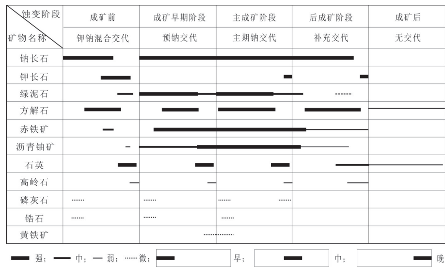
图 4 菱岭矿床钠交代蚀变似斑状花岗岩中矿物共生关系 Fig.4 Mineral paragenesis in Na-metasomatic porphyritic granite of the Jiling uranium deposit
