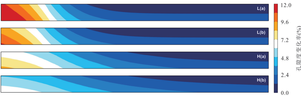
图 7 1 500 d 时储层孔隙度的空间变化 Fig.7 Spatial variation of porosity of the reservoir at 1 500 days y轴放大 5 倍
