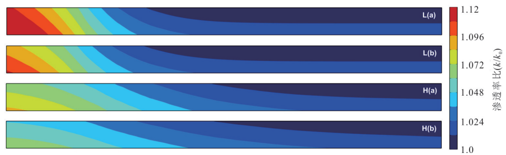
图 8 1 500 d 时储层渗透率的空间变化 Fig.8 Spatial variation of permeability of the reservoir at 1 500 days y轴放大 5 倍
