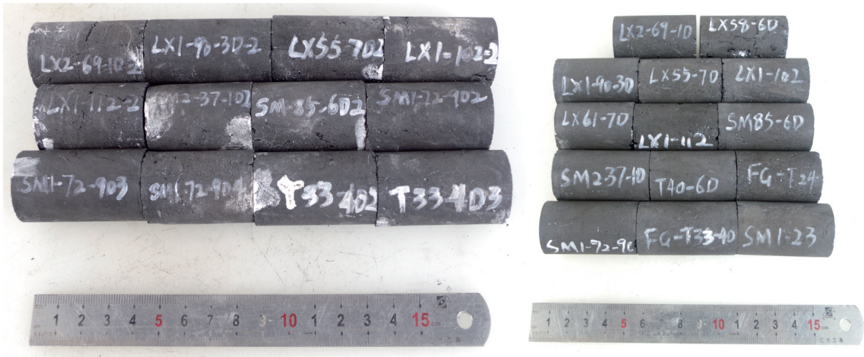
图4 试验所用标准岩心柱样品 Fig.4 Representative standard core plug samples utilized in the testing
