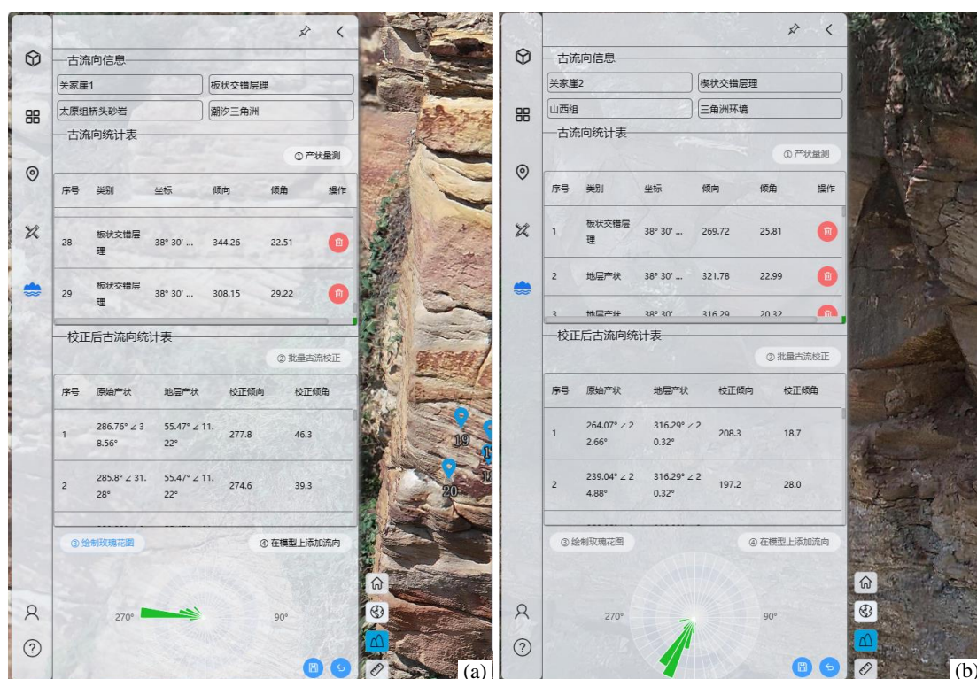
图 11 关家崖露头 1 (a) 太原组某一层位、露头 2 (b) 山西组某一层位古流向玫瑰花图 Fig.11 Paleocurrent direction rose diagrams of a certain stratigraphic horizon of the Taiyuan Formation in Guanjiaya outcrop 1 (a) and a certain stratigraphic horizon of the Shanxi Formation in Guanjiaya outcrop 2 (b)
