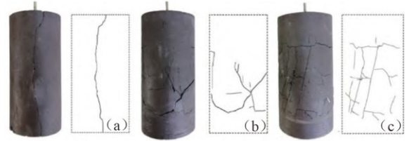
图 3 (a) 水力、(b) 液态 CO 2 、(c) 超临界 CO 2 压裂后煤岩表面裂缝形态(改自梁卫国等, 2022) Fig. 3 Fracture morphology of coal surface after (a) Hydraulic, (b) liquid CO 2 , and (c) supercritical CO 2 fracturing (modified from Liang et al., 2022)
