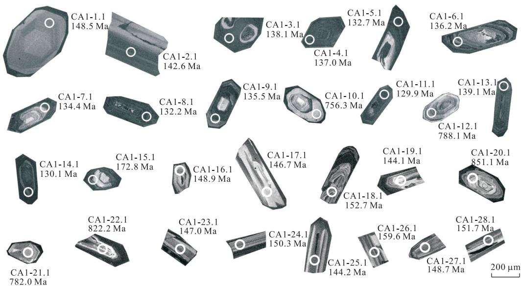
图6 大铜坑花岗岩锆石的阴极发光图像及SHRIMP分析点位和 $^{206}\text{Pb}/^{238}\text{U}$ 视年龄Fig.6 CL photomicrographs, measured points and age data ( $^{206}\text{Pb}/^{238}\text{U}$ ) of zircons from the Datongkeng granite
