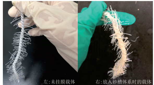
图 3 挂膜前和挂膜后的生物载体 Fig.3 Biological carriers before and after membrane hanging
